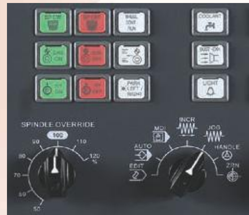
A light has been added to ensure ease of spindle speed monitoring at 100% spindle override position.
